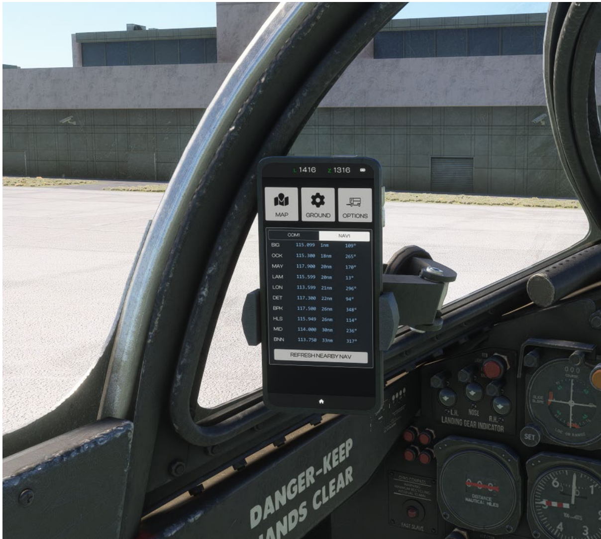
Home Page (incorporating local NAV1 VOR Frequencies. This feature will also automatically tune the NAV1 radio when the frequency is selected)
