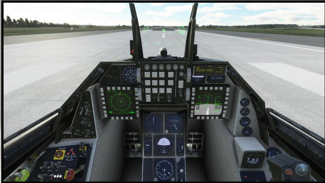
The cockpit of the F-16A Fighting Falcon is a mixture of Multi-Function-Displays common to many modern aircraft, and analogue gauges reminiscent of the aircraft's design era, the 1970s. The cockpit is surprisingly small compared to many fighter aircraft as a result of weight-saving considerations during its design, and the pilot sits quite high above the canopy sill, increasing visibility further through the large teardrop-shaped canopy.
