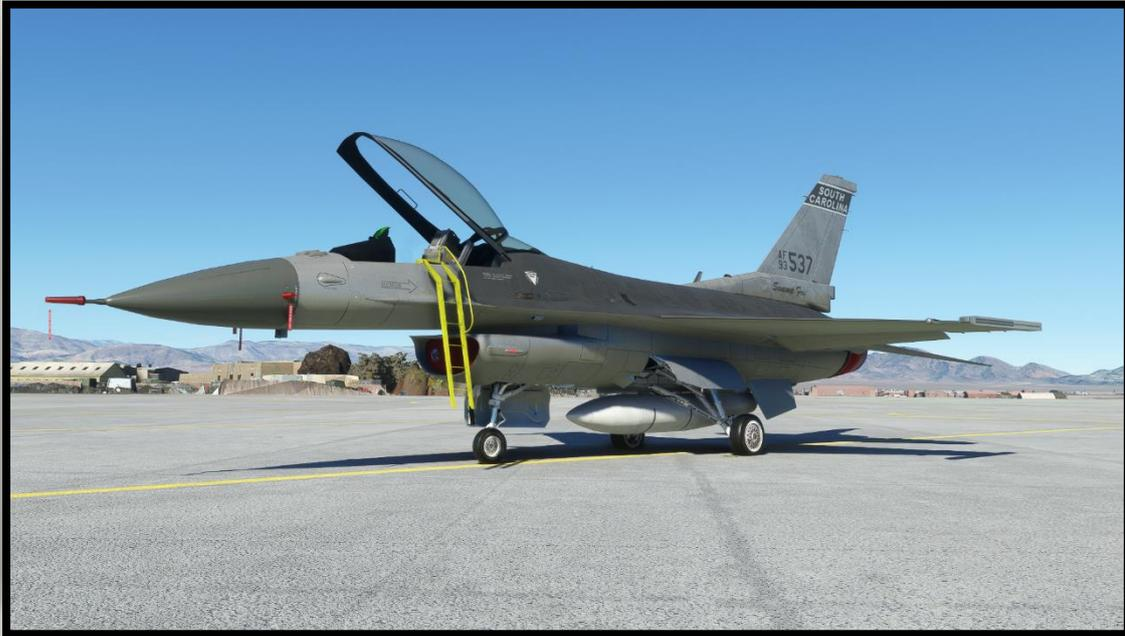
If you're starting from cold-and-dark, on the apron, you will find that the aircraft will have its chocks and covers deployed. The F-16 Fighting Falcon is fitted with an Auxiliary Power Unit, so engine-start is a fairly straight-forward procedure with no ground power option required.
