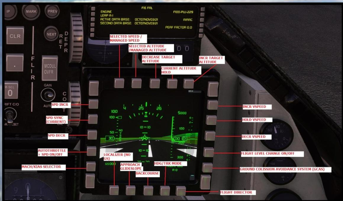
1. **SEL/MNG SPEED TOGGLE:** allows you to select between managed or selected speeds for use with auto-throttle. Default mode is “selected airspeed”, allowing to increase / decrease the speed manually by using the spd + spd- keys. Managed speeds
