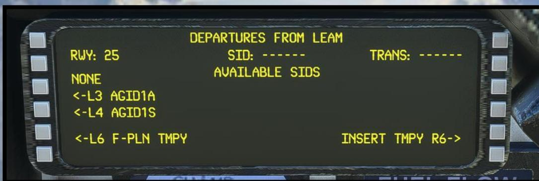
For this example, we will select AGID1A, by pressing L3 Button, we can also select SID if available, otherwise press R6 to insert the procedure and update the FlightPlan.
