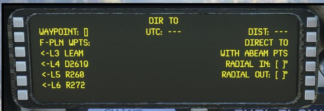
Direct TO mode allows the user to enter an Airport by ICAO format to trace the direct route from current position to a desired destination either if you have or not a created
