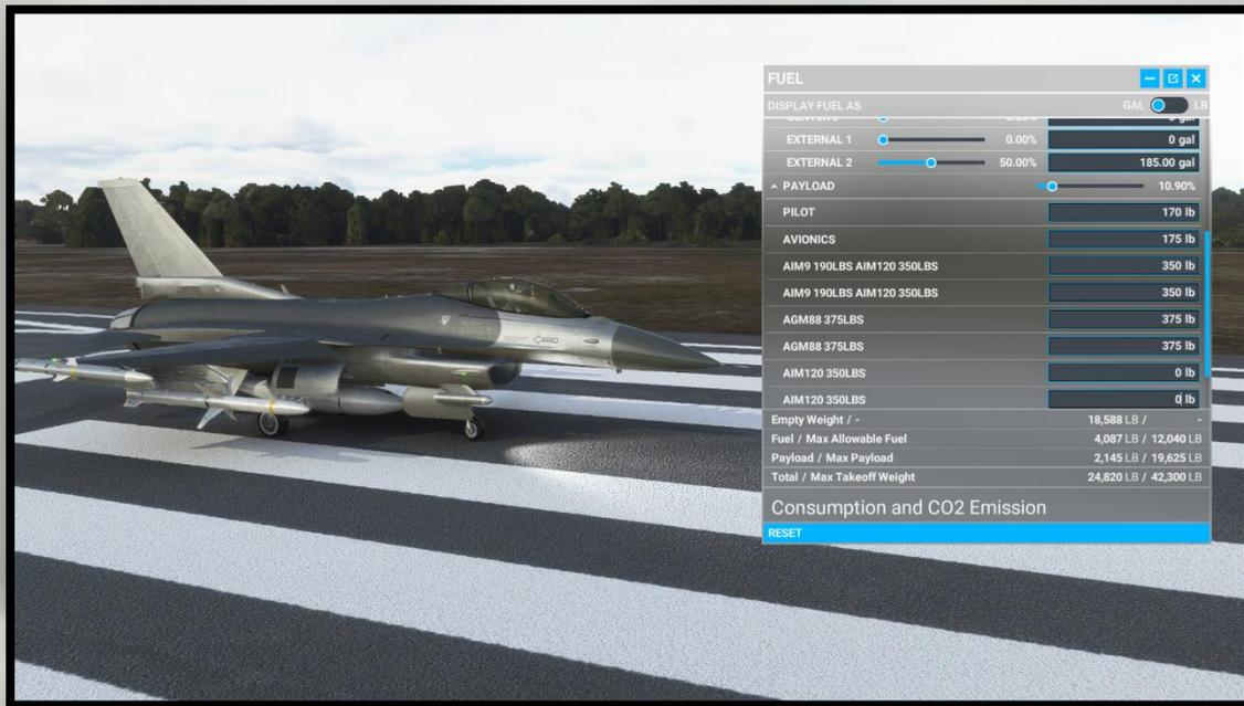
In the above image, the pilot has selected external tanks with 50% fuel in each, has internal fuel ( just out of the menu shot in tanks CENTER 1 and 2 ) and has also loaded AIM-9 *Sidewinder* missiles and two AMRAAM medium-range missiles, by typing in the relevant weights as listed in the stations on the right of the menu. Total weight is 24,820 with 4,087lbs of fuel aboard.
