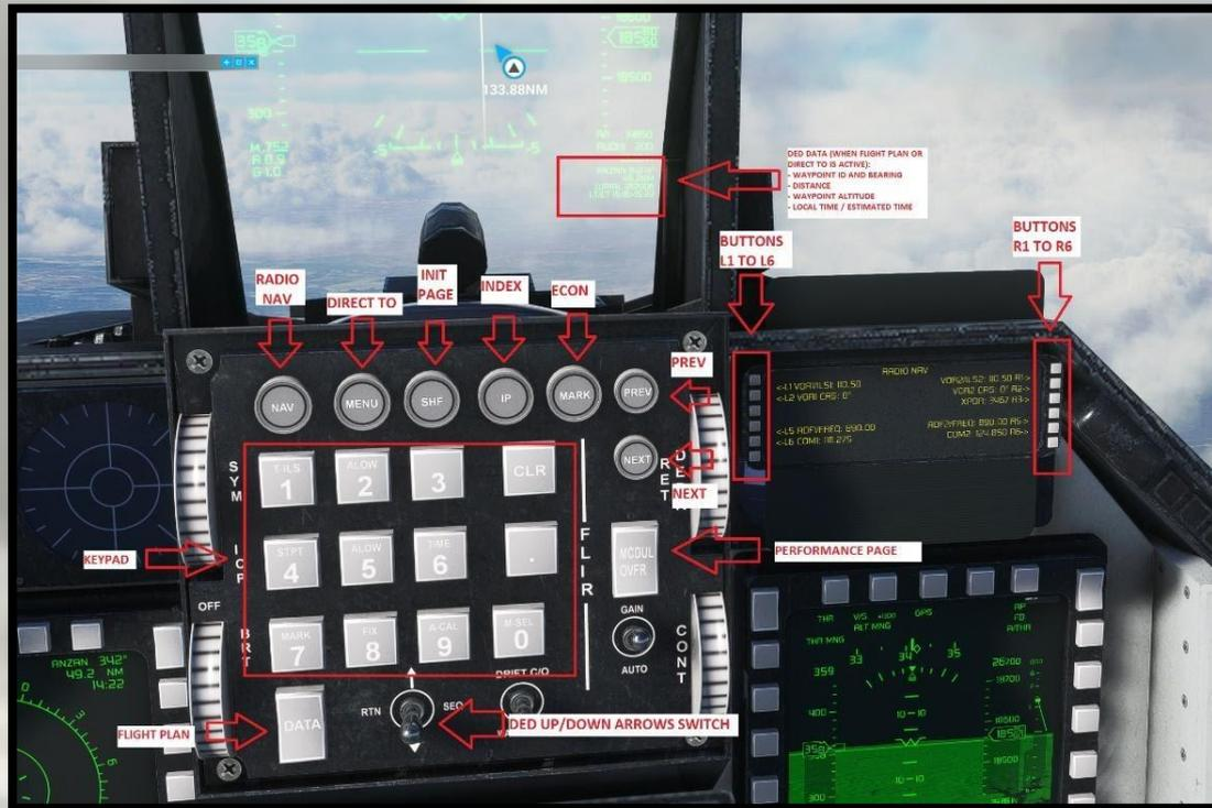
Unlike the real DED, in which we use the numeric keys to navigate through the different DED menus, in this case the keypad has been provided with alphanumeric capability (like old phones alpha numerical Keypad Style) to be able to store different data into the console, from VOR/ILS or COMMS frequencies, to airport codes in ICAO format to be able to create flight plans, or simply use the direct TO mode.
