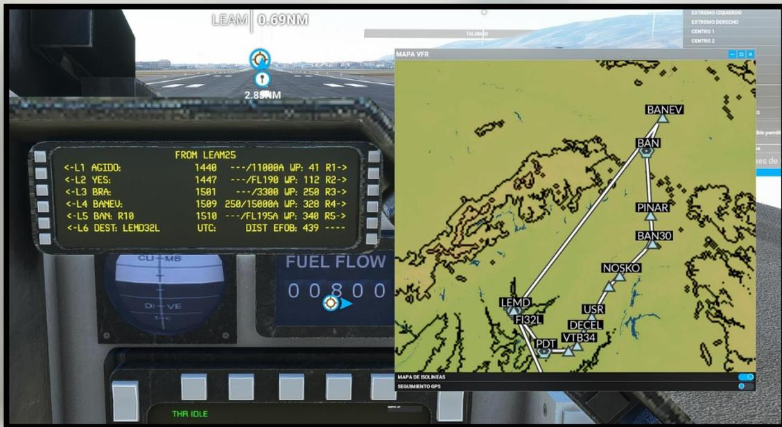
However, I recommend to fix a bit the procedure, in this case I will erase from the procedure the Waypoint BRA, by pressing CLR, followed by L3 to erase BRA:
