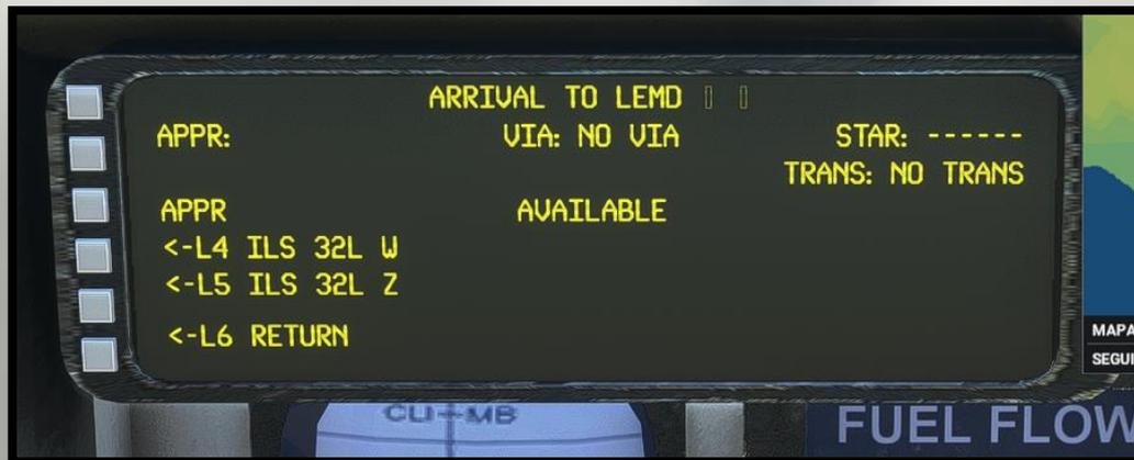
We can also select an available VIA and STAR if desired, for this example, we will choose ASBIN as VIA, and BANE2D as STAR. After finish, we will store the procedure in the FPLN by pressing R6:
