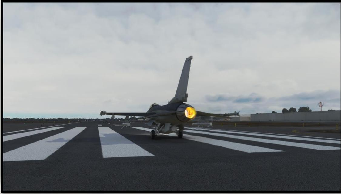
The F-16A Fighting Falcon rotates at around 120 knots, with the nose up at ten degrees and held there until the aircraft “unsticks” itself from the runway. Gear retraction should be brisk as the aircraft will accelerate rapidly in full afterburner. The aircraft’s auto-trim system will engage above 245 knots to assist the pilot in precision control, while the flaps and slats will retract automatically.
