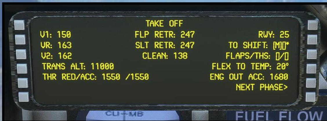
Performance pages display the performance parameters for the current flight phase. They are automatically sequenced after the take-off phase.
