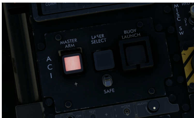
ACI Panel, note MASTER ARM on. Press BUOY LAUNCH to deploy
