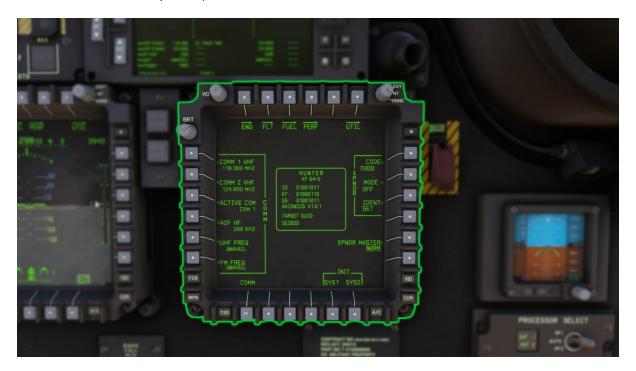
On this page you will see the communication panel, where you can see and set COM and NAV frequencies. Frequency input follows the Keyboard Panel Interaction system and allows you to change the active frequencies for COM1, COM2, ADF, and the transponder (XPNDR) code.
