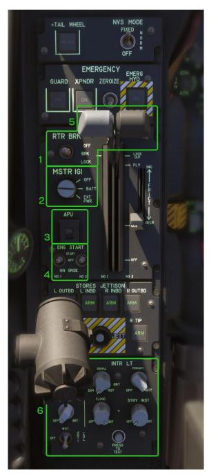
o LOCK OUT: When the lever is moved to this position, the system will enable the MANUAL mode, which will adjust the power according to the lever position between idle and lock out position. This mode will be always activated until you move the throttle lever to IDLE again and set it to FLY
