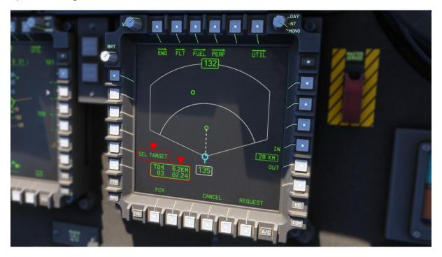
The Diamond Indicator will correspond to the target's position within a 3D virtual environment, synchronized with the FCR page and the target's dotted line. This ensures that you can locate the targets in an efficient manner and strike accurately!
