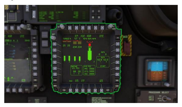
The **ENG** sub-page displays several indicators from the engine and hydraulic systems. The most important readings are **Torque**, **NG**, and **NR**.
