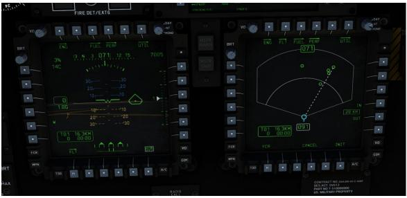
Both the FCR and FLT pages feature a TARGETS window in the bottom-left corner, displaying the next target index (T01 to T08), their distance from you, your ground speed, and the estimated time to reach it at your current speed. If you wish to cycle between the targets, press the softkey next to "SEL TARGET" this will select the next available target and adjust the current track and update the target information window to the relevant data.
