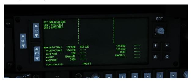
Press the "P" key to enable edit mode. This will display a green square to the left of the selected value, indicating it is ready for editing. Enter the desired value using the numeric keypad. Note that the message code now includes the EUFD suffix. After entry of the desired value, return to the EUFD, verify that the green square is active, and then press the ENTER key (4). Then verify that the value has been updated.
