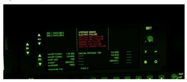
Every time a new RED message is displayed, the system will trigger the MASTER WARNING alert. This can be identified by the illumination of the MASTER CAUTION button or by an audible alert, which can be silenced by pressing the button.
