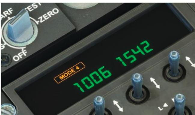
Move the FUNC switch down twice more to select the Mode S flight ID display page. Here you can set an alphanumeric flight ID for use with Mode S, using the same method as for editing the transponder codes.
