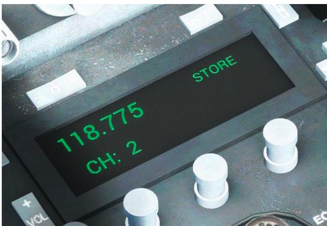
The display will revert to manual mode and the new frequency preset will be shown on the frequency cards in channel 2.
