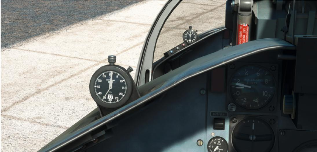
A stopwatch is fitted to the left frequency card in both cockpits.
