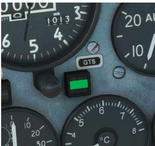
Set the engine start switch to **START** and release. The engine will begin to spool up and, once the rotation indicator shows green and the RPM has reached approximately 15-20%, click on the throttle idle stop lever to advance the lever to the **IDLE** position.
