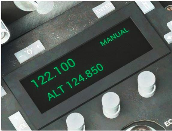
The active COM 1 frequency can be stored as one of 20 preset channels. Press the MENU push-button to enable or disable store mode, as indicated by STORE on the LCD. The navigation rocker switch is used to select the desired preset channel (1-20) and the ENTER push-button is used to store the frequency.
