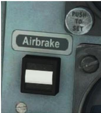
Push the airbrake switch forward to the **IN** position before releasing it. Confirm that the Airbrake indicator on the left instrument panel shows black, indicating that the airbrake is retracted.
