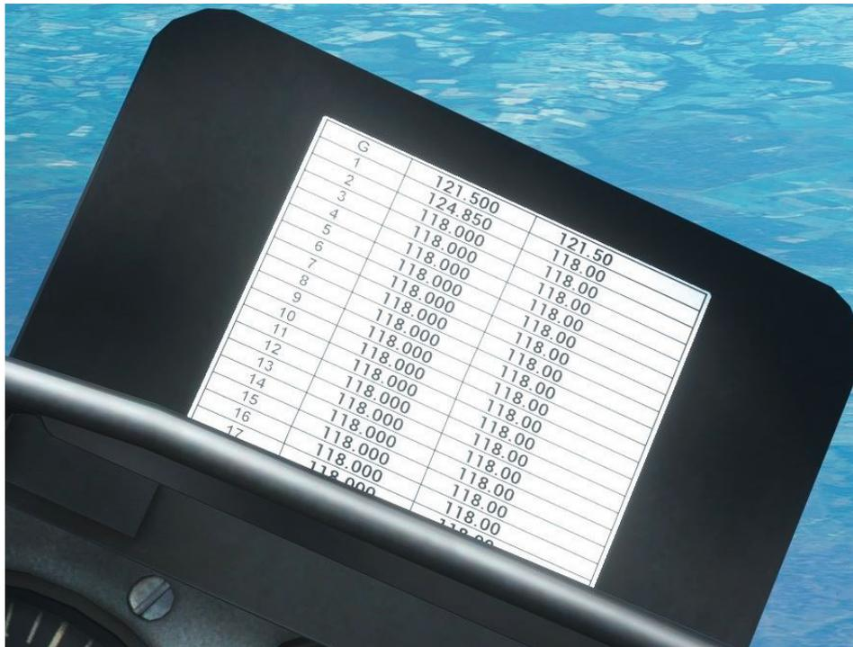
If you return to the manual mode by rotating the frequency mode selector to the **MAN** position, you will see that the preset frequency has now been tuned as COM 1 standby, shown in the lower portion of the display. To make the frequency active, press the **ENTER** button.
