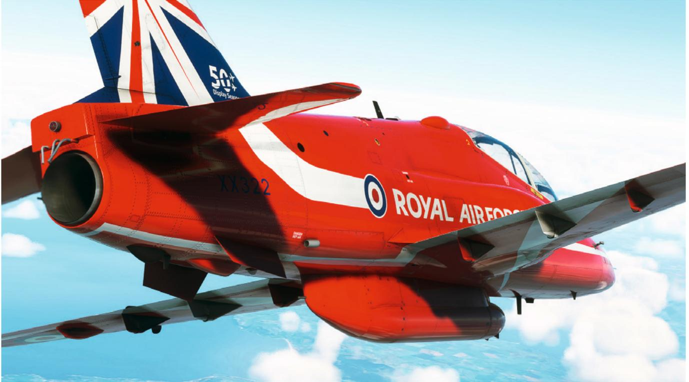
Aerodynamically, the aircraft is of conventional design with a moderately swept wing with a 2° dihedral and trailing edge double-slotted flaps. A one-piece all-moving tailplane is swept back and has a 10° anhedral.
