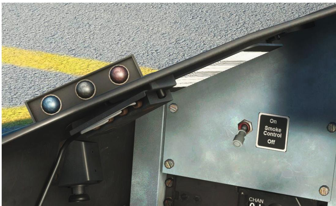
With the Red Arrows configuration selected, the aircraft will be equipped with the centreline fairing for carrying display smoke diesel fuel and dye, and associated cockpit controls.
