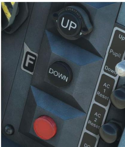
A red landing gear selection control transfer button is fitted to the rear cockpit only.
