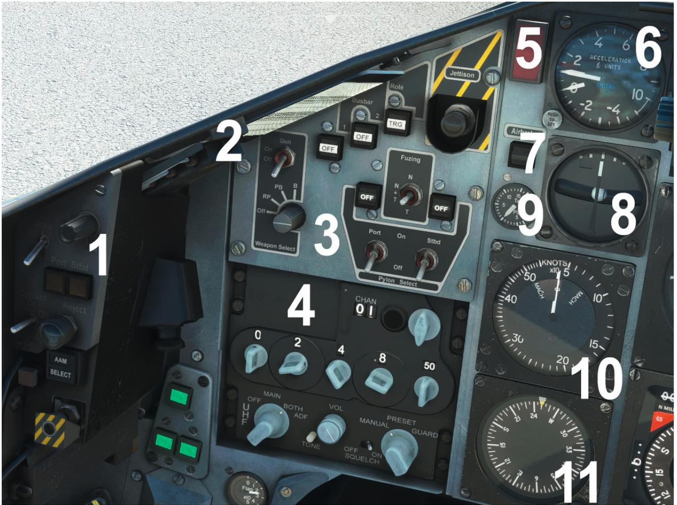
1. Missile (AIM-9) control panel (only visible when T1/A configuration selected)
