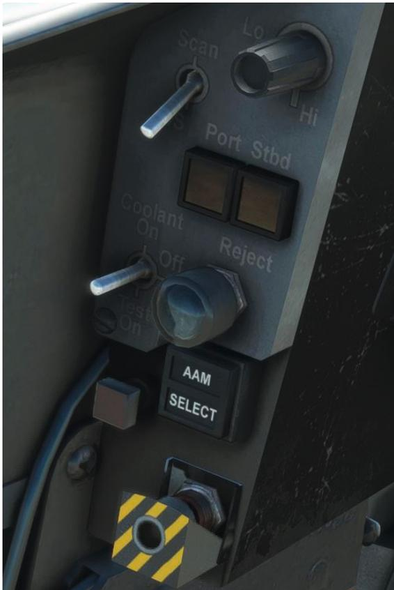
Sidewinder AAM can be carried on a launcher installed on each of the pylons. The MCP enables either of the missiles to be selected for firing and both missiles to be jettisoned by launching as a pair in an inert state.
