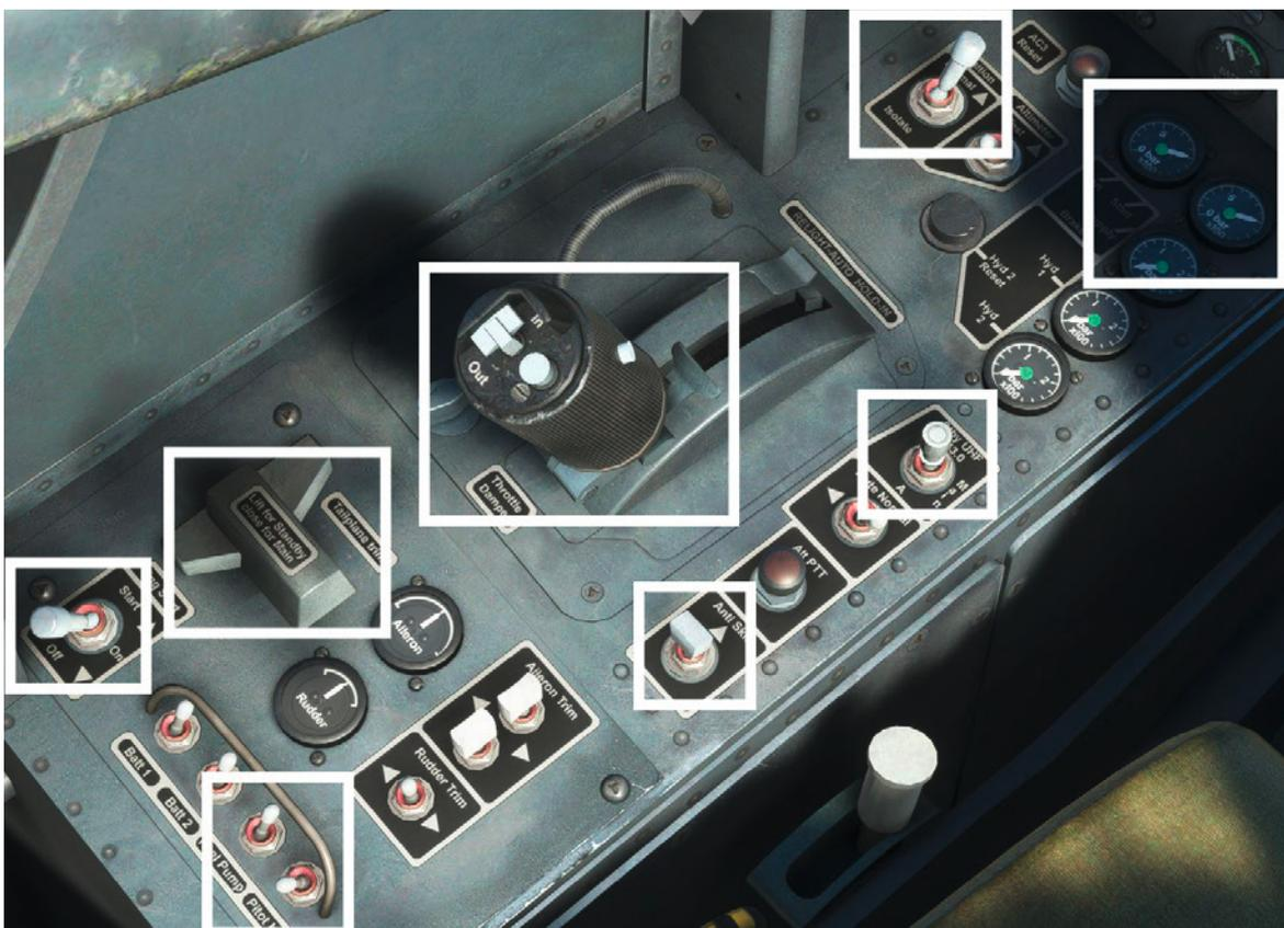
Moving up to the left instrument panel, confirm that neither the U/C (undercarriage – gear) or flap standby handles have been pulled out.
