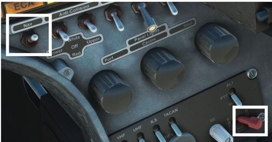
Finally, confirm that the parking brake handle is pulled to **ON**. The handle is located at the aft end of the right console.
