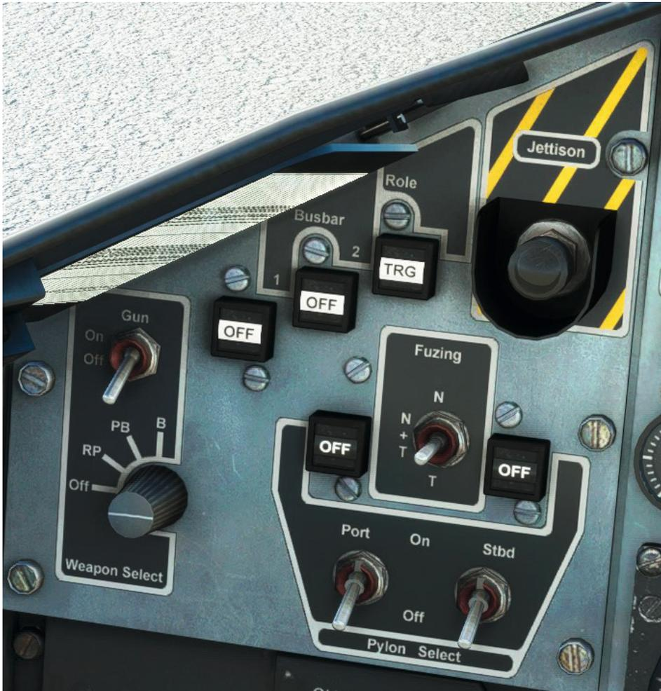
The WCP allows for the selection of any pylon-loaded store, except Sidewinder missiles, for release or the gun for firing. The WCP also allows pylon-loaded stores, except Sidewinders and their launchers, to be jettisoned.
