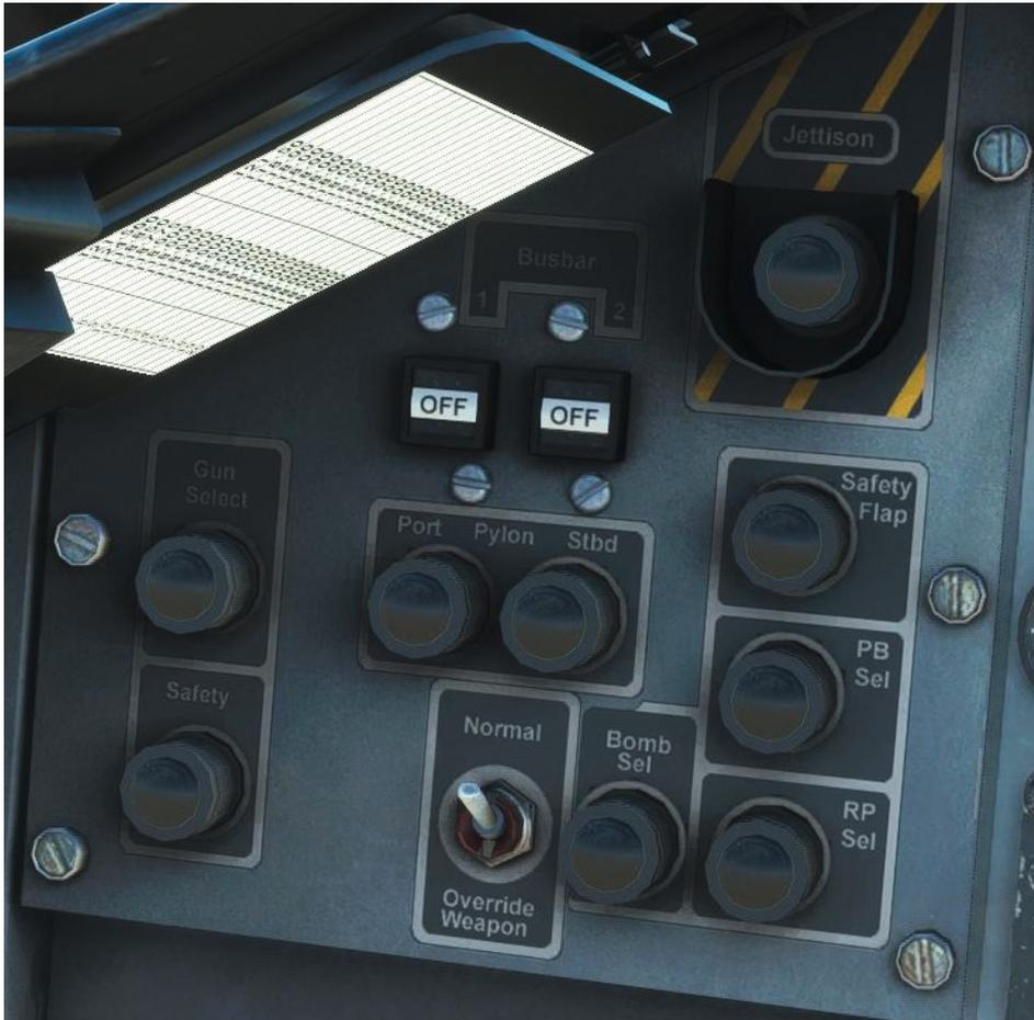
When the rear cockpit main lights master switch is on, the WMP is lit by the strip light below the glareshield; the power MI are then integrally lit.
