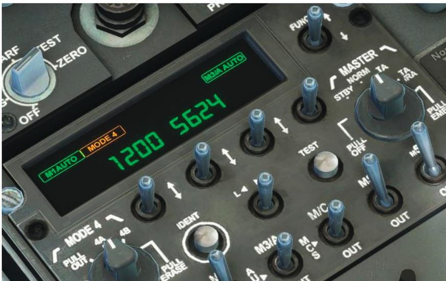
MSFS has limited transponder capability and only civilian modes are supported, so only the Mode 3/A (right) code serves a purpose, although you can edit both to simulate real-world operations. We will now edit the Mode 3/A code.
