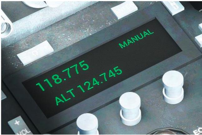
Now press the **MENU** button to enable store mode. Using the navigation rocker switch, select channel 2 (CH: 2) and then press the **ENTER** button to save the COM 1 active frequency into preset channel 2.
