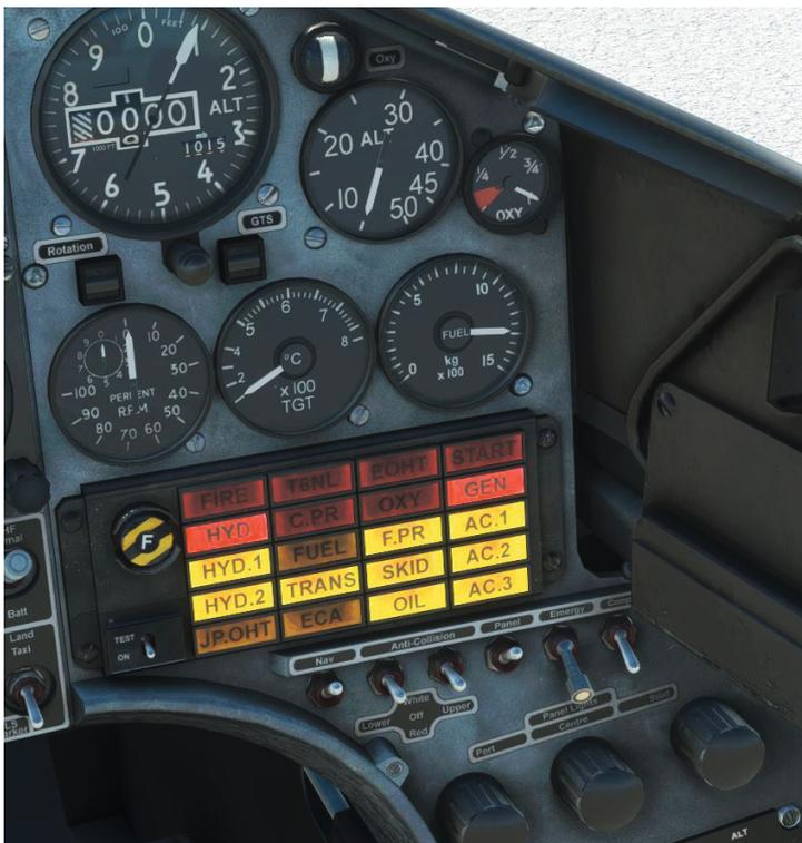
Moving across to the right instrument panel, confirm that the OXY CWP caption is off, the oxygen contents are over 1/2 full and the flow indicator shows oxygen flow.
