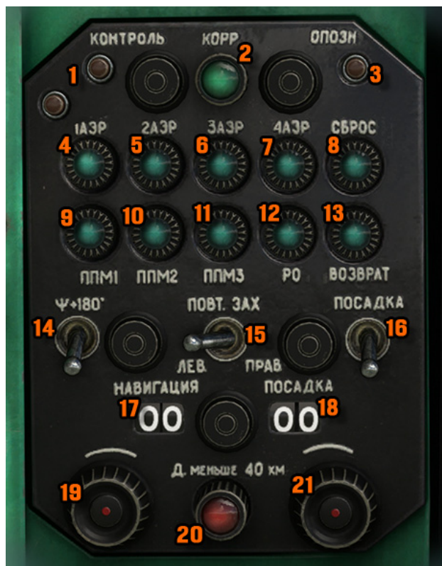
Fig. 48 - RSN (Radio Navigation System, SHORAN)
