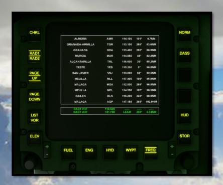
The Radio (FREQ) format, shows the V/UHF frequencies for the two manual channels and the 24 variable frequencies in a radius of 200NM shown on pages of 12. The data presented is based on three categories: VOR (VHF), ARPT (UHF) and NDB (ADF). This format is only limited to displaying information. Well, the frequency tuning is done through the central knobs, the HDD or the DEP under the MDE RAD1 and RAD2 submenus.
