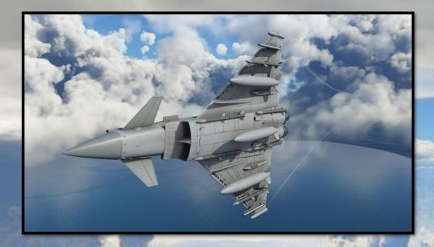
The Eurofighter Typhoon rotates at around 120 knots, with the nose up at ten degrees and held there until the aircraft "unsticks" itself from the runway. Gear retraction should be brisk as the aircraft will accelerate rapidly in full afterburner. The aircraft's auto-trim system will engage above 240 knots to assist the pilot in precision control, while the flaps and slats will retract automatically.
