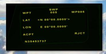
3. Press DN key to select LON and enter the coordinate in the format E000000000 or S000000000, and press enter:
