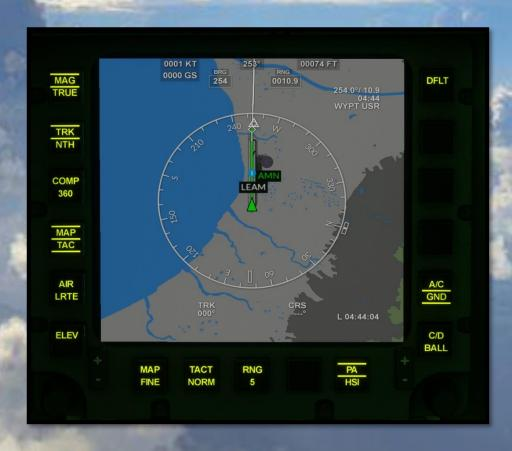
The Horizontal Situation Indicator (HSI) format, displays the following TACAN or navigation system derived data:
