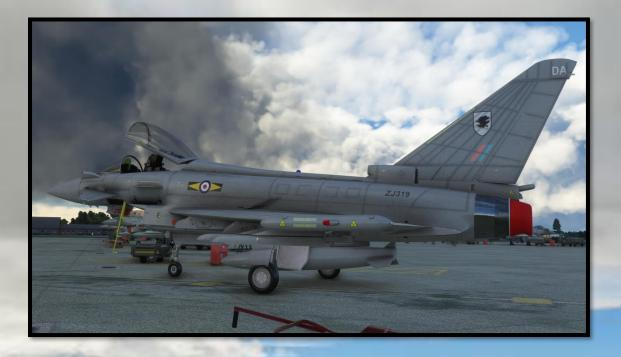
The Eurofighter Typhoon employs the classic lines of a delta-canard and a modern fly-by-wire system that gives the aircraft its tremendous manoeuvrability. Although a naturally unstable configuration, complex calculations by the on-board computers correct for this instability, with the pilot then able to fly the aircraft in a relatively "carefree" manner, essential in a close-combat environment where airspeeds and even altitudes can become dangerously low.
