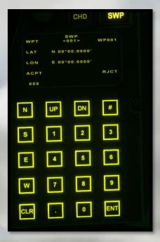
2. Press DN key to select LAT and enter the coordinate in the format N00000000 or S00000000, and press enter:
