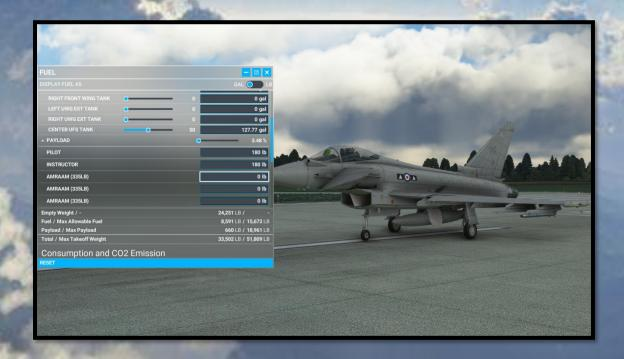
In the above image, the pilot has selected external centreline tank with 50% fuel, has internal fuel (just out of the menu shot) and has also loaded ASRAA missiles by typing in the relevant weights as listed in the stations on the right of the menu. Total weight is 24,251 with 8,591lbs of fuel aboard.
