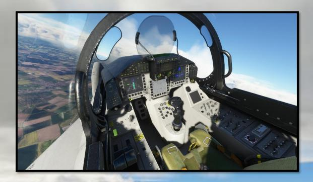
The cockpit of the Eurofighter Typhoon is dominated by Multi-Function-Displays common to many modern aircraft.
