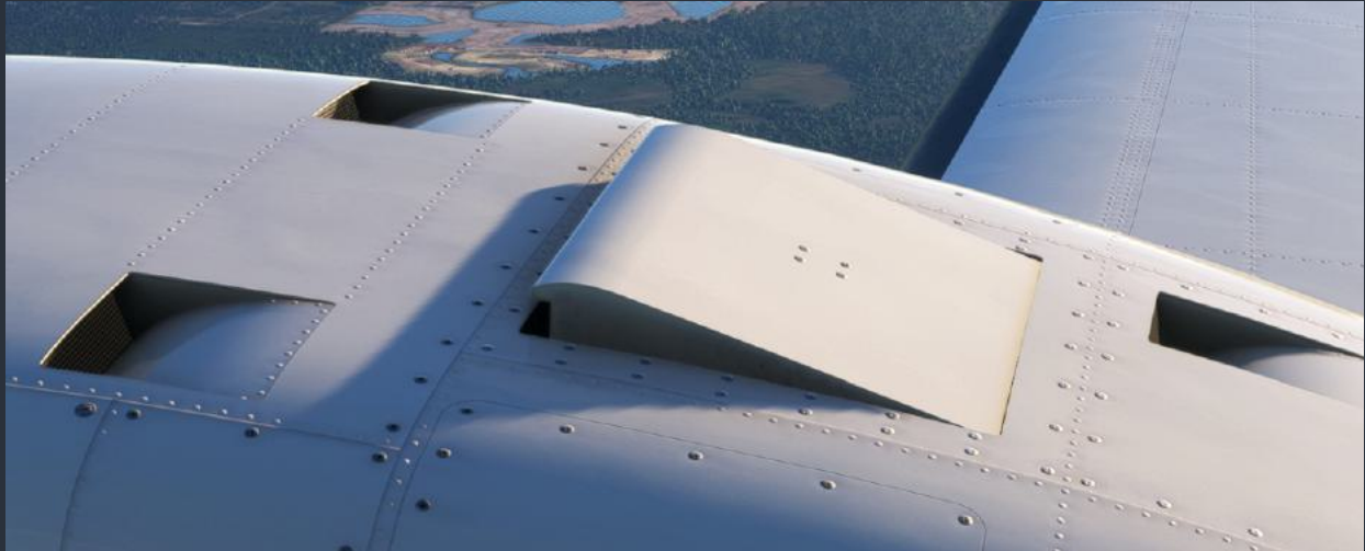
Above: pressurization intercooler door, partially extended - flight position
