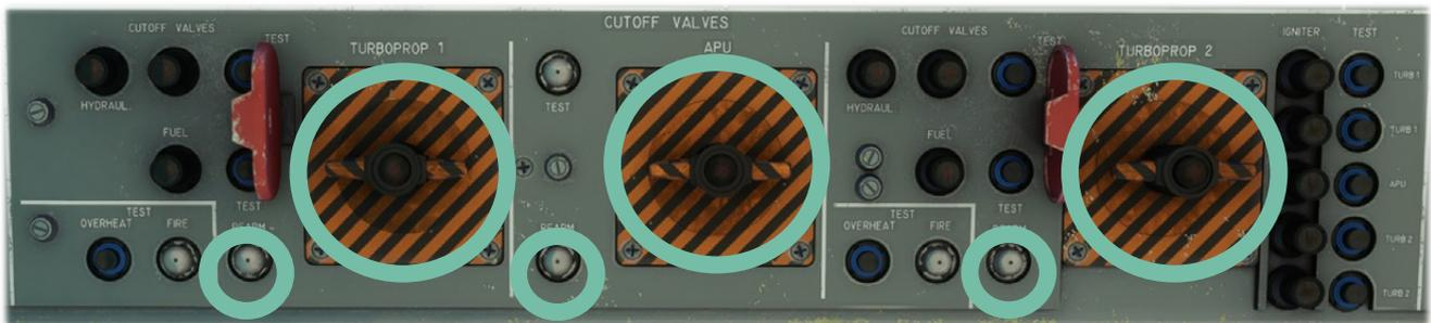
Main engine valves do not have any manual handle but are automatically closed when condition levers are put in shut-off position.
