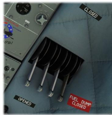
In case of engine fire, a cut-off valve directly located nearby the engine (or APU) can isolate the concerned engine or the APU from the rest of the fuel system.
