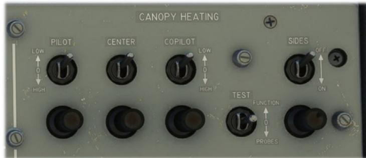
Each zone has a light which is on when heating is not functioning.
