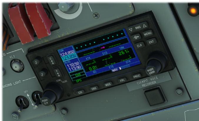
As described in autopilot section, GPS route can be automatically followed by the autopilot in radio mode.
