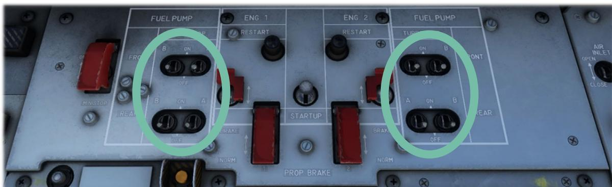
Those pumps should be functioning from the takeoff until landing to ensure a sufficient fuel pressure.
