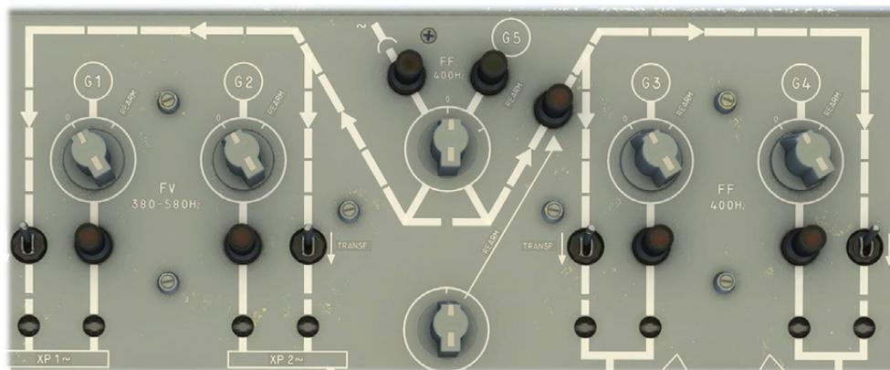
When APU nominal RPM value is reached, G5 generator is available. In this case it can be selected using GPU/G5 selector knob. A green light turns on when G5 is selected.
