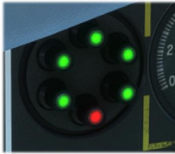
A red light will glow if landing gear is not down and locked while airspeed is below 115 knots and throttle position is low.
