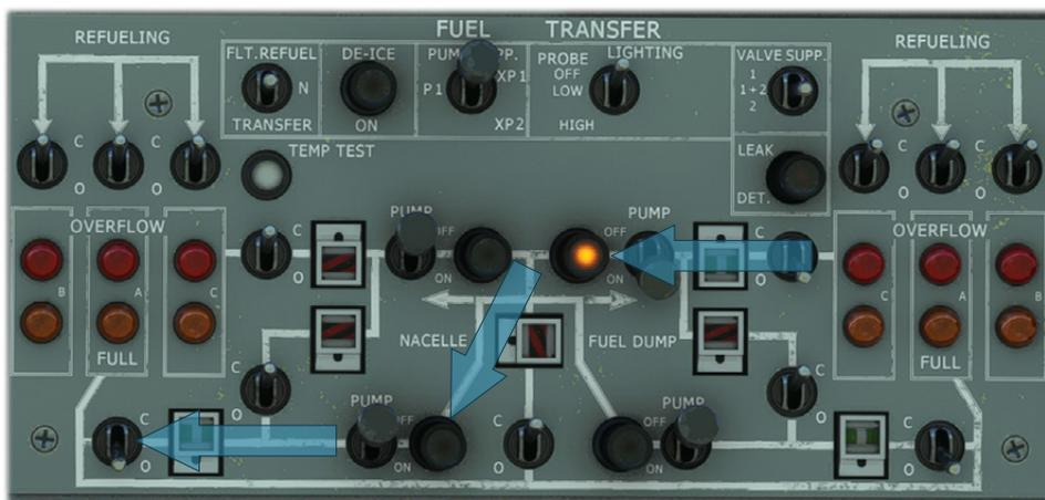
To dump fuel, valve associated to the tank to drain should be opened, and the associated pump turned on. Opening fuel dump valve handle will initiate fuel dumping.
