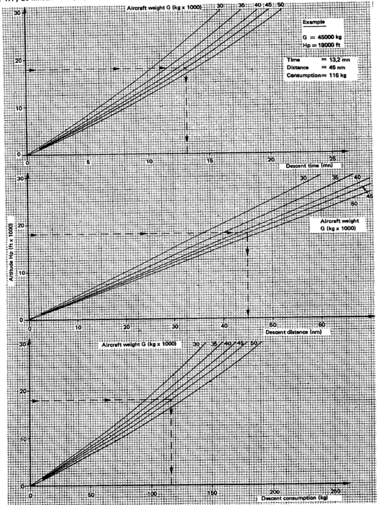
**RAPID DESCENT** Airbrakes fully extended – Reduced engine power – L.S.A. – C.A.S. = 180 kt
