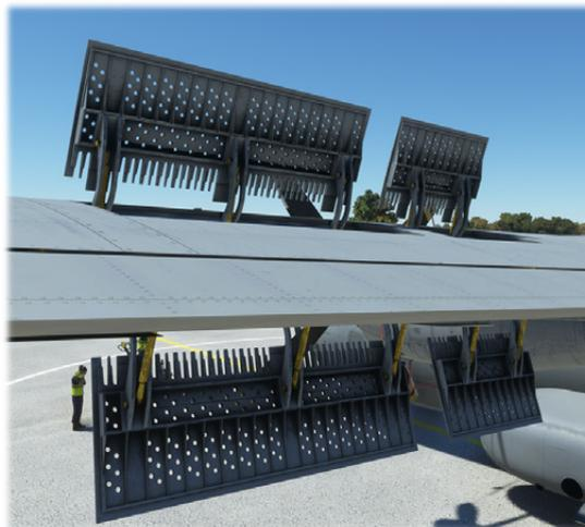
In case of hydraulic failure with spoilers extended, an emergency lever allows to retract them.
