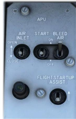
Air inlet needs to be opened prior to starting the APU as it allows air supply. Starter switch will trigger an automatic sequence after which APU will reach and maintain 100% RPM.
