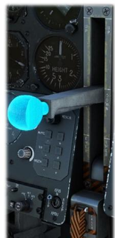
A set of five green lights indicate that landing gear is down and locked (front landing gear and each axle of main landing gear). Red light indicates that landing gear and hatches are maneuvering and not locked.
