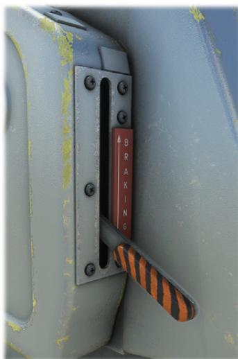
An anti-skid system, called "ministop" is enabled from center console. It is automatic and will minimize braking distances depending on wheels rotation speed and ground adherence.
