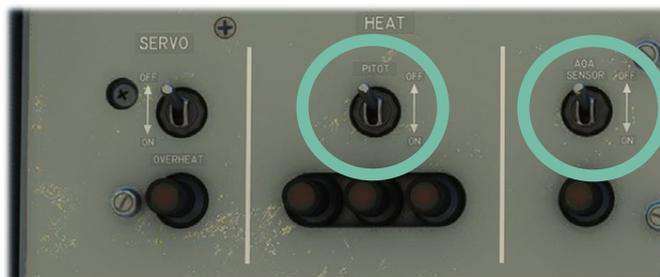
It can normally be heated up in order for the crew to visualize the speed of ice formation on it. This functionality is not simulated for now because of technical limitations. However, the tube can be lighted from the de-icing panel.
