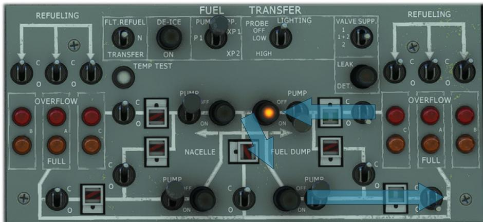
In the following configuration, fuel will be pumped out of right tank C to be transferred to left tank A:
