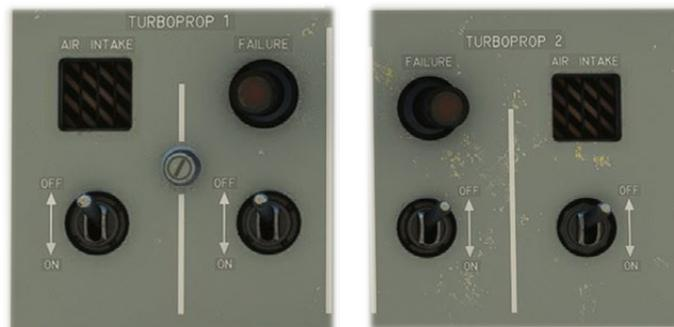
Propeller de-icing works the same way as airframe de-icing but only with cycled heating.
