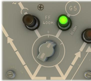
On each generator circuit, a red light indicates either a failure or a loss of power.
