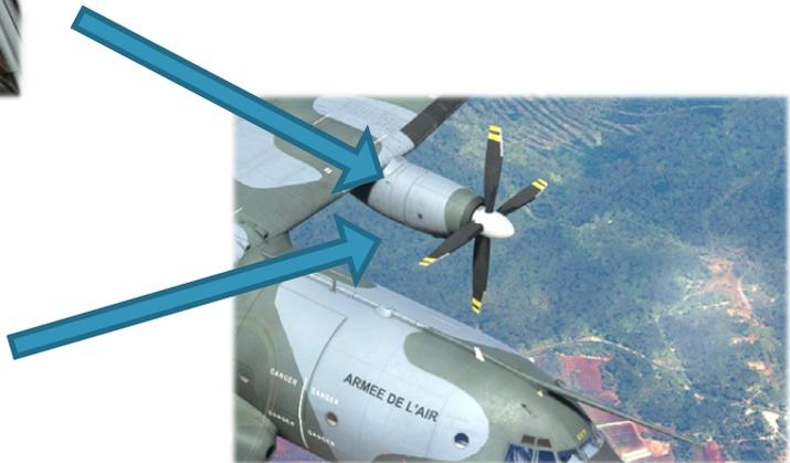
While on-ground with engines off, an electrical motor can be used to put propeller in feather position:
