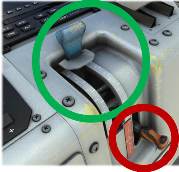
In case of hydraulic failure on the main (green) circuit, an emergency lever is available to operate flaps using red hydraulic circuit.
