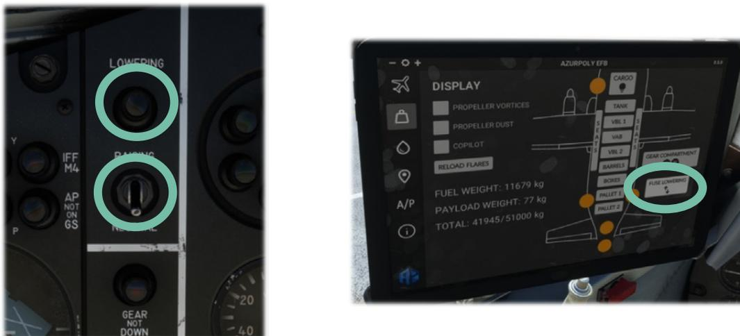
Front panel switch can only raise the fuselage. In the real aircraft, lowering is not automated and must be carried out by an operator on a dedicated panel in the cargo bay.
