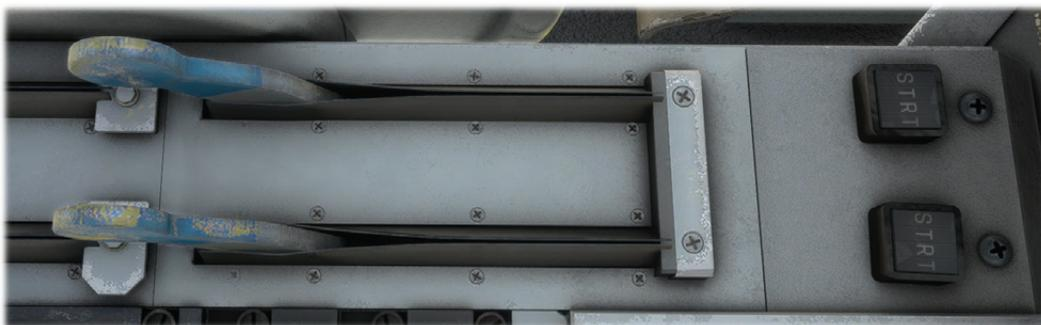
Idle lever purpose is to control fuel injection during engine startup. They have two positions:
