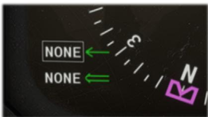
Heading reference bug represents target heading and will be used by the autopilot when it is running in heading selection mode.
