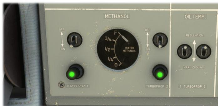
Once pumps are running, injection will start only if condition levers are fully forward and if engine torque is above 75 PSI.
