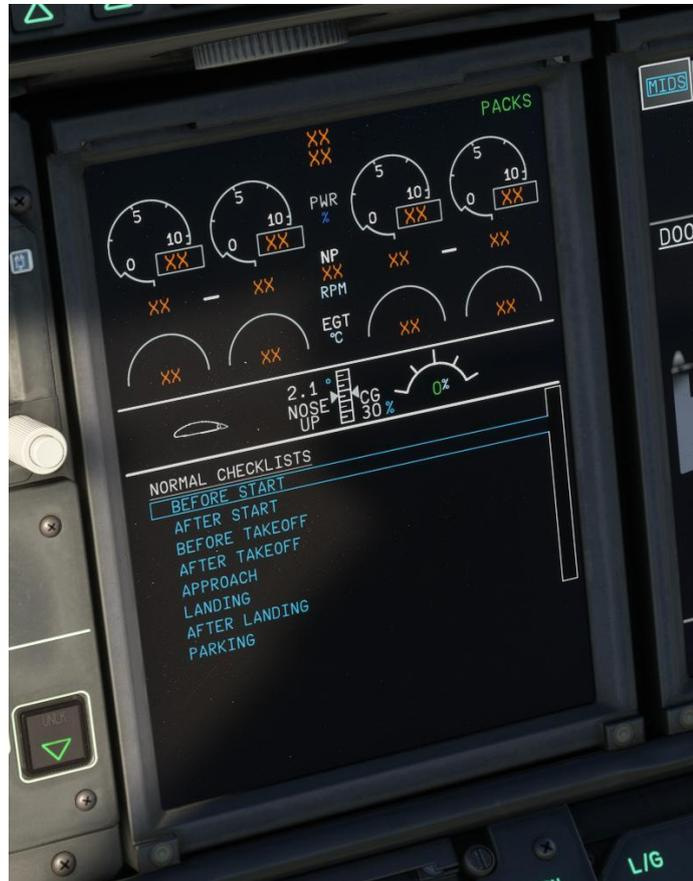
Items that require manual intervention are preceded by a tick box () , press the ECAM Check button to proceed to the next item.
