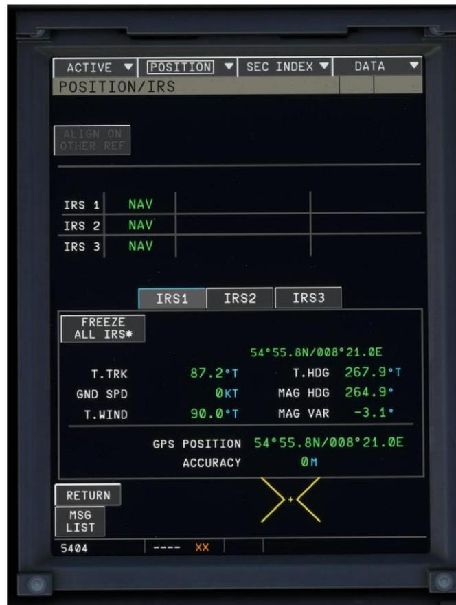
Check that the IRSs are all aligned and the position is correct. Press RETURN.
