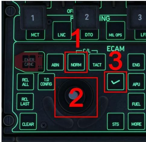
Using the Pedestal Joystick (2) you can scroll up or down to select a different checklist or checklist item. When the required item has been highlighted, press the ECAM Check button (3) to access the checklist.
