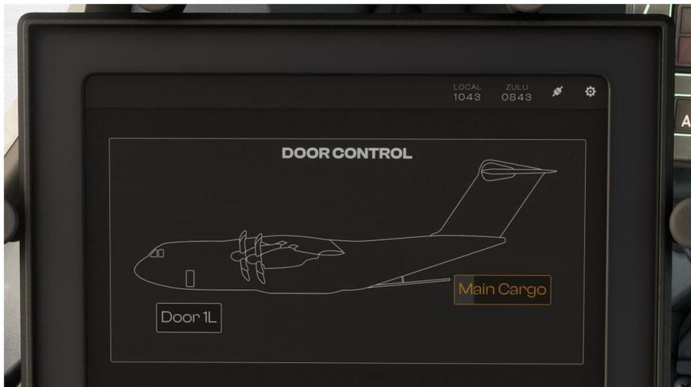
Once the door is open (or closed), turn the Blue Hydraulic Electric pump off by lifting the guard and pressing the ON push button.
