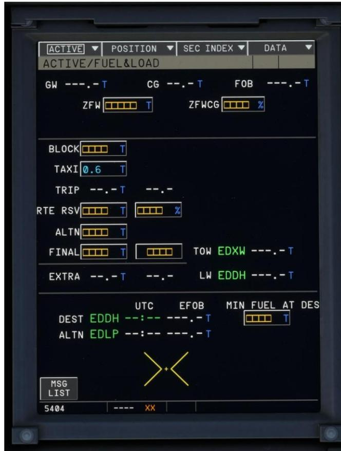
Insert your ZFW, ZFWCG and BLOCK fuel as displayed in the EFB Fuel & Payload page. When you are done, press PERF in the KCCU to access the performance page.
