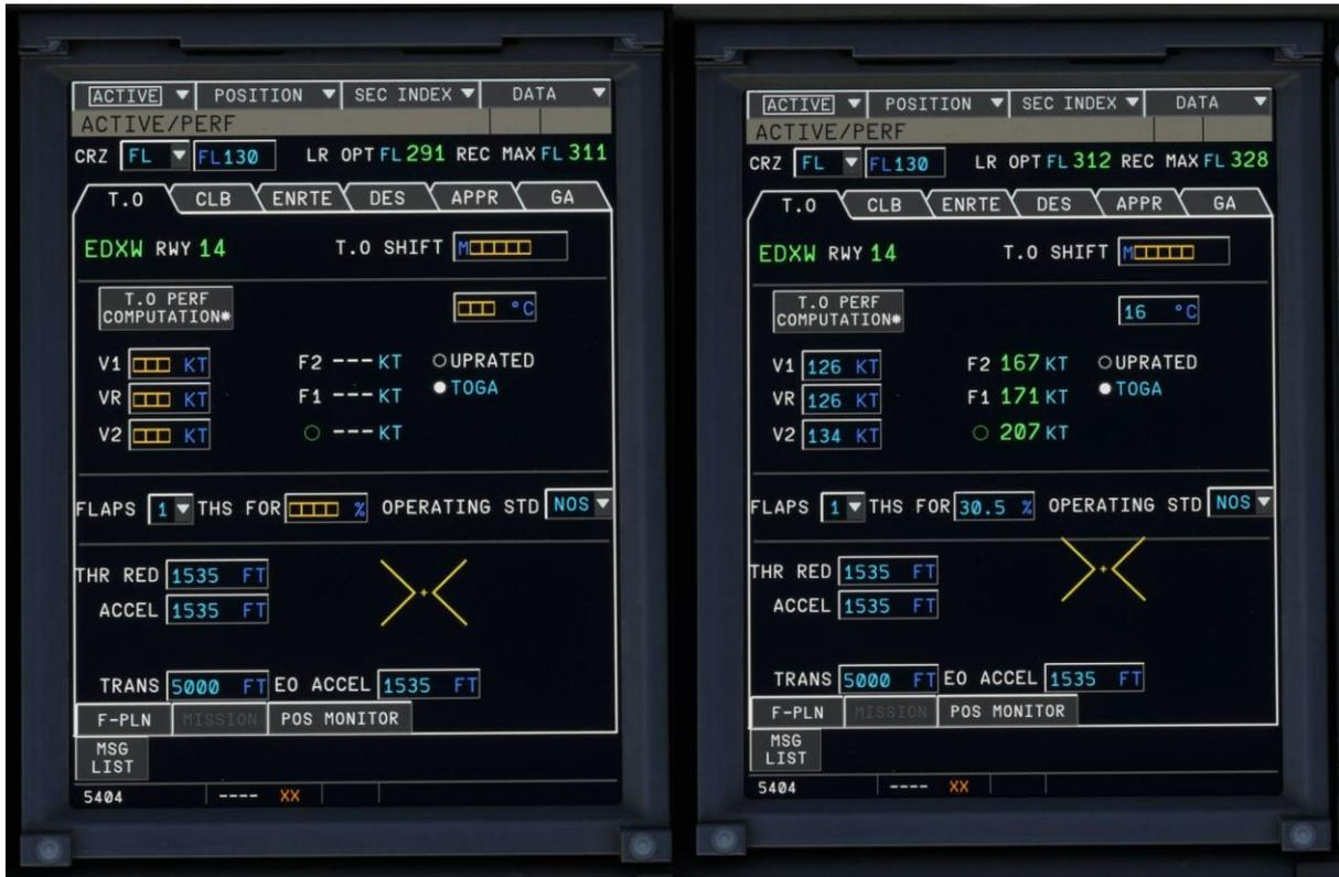
Press T.O PERF COMPUTATION\* to automatically calculate and insert your take off speeds and trim setting.
