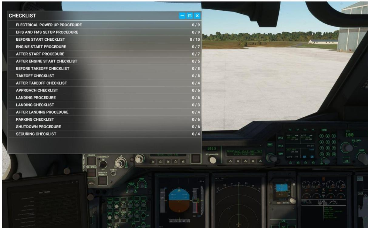
Clicking the blue eye icon to the right of the checklist item will switch your view to the requisite panel where the button/switch/dial/gauge is located. You can use the AUTO COMPLETE option to expediently tick off the item from the checklist.
