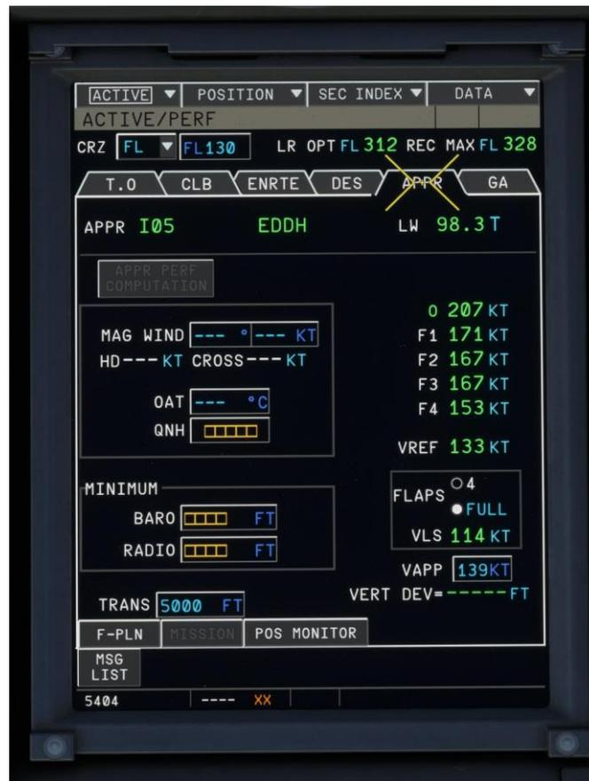
Pressing the APPR button will display the Approach page. Here is where you will insert your weather information, applicable minima and be able to see your minimum configuration speeds and approach speed.
