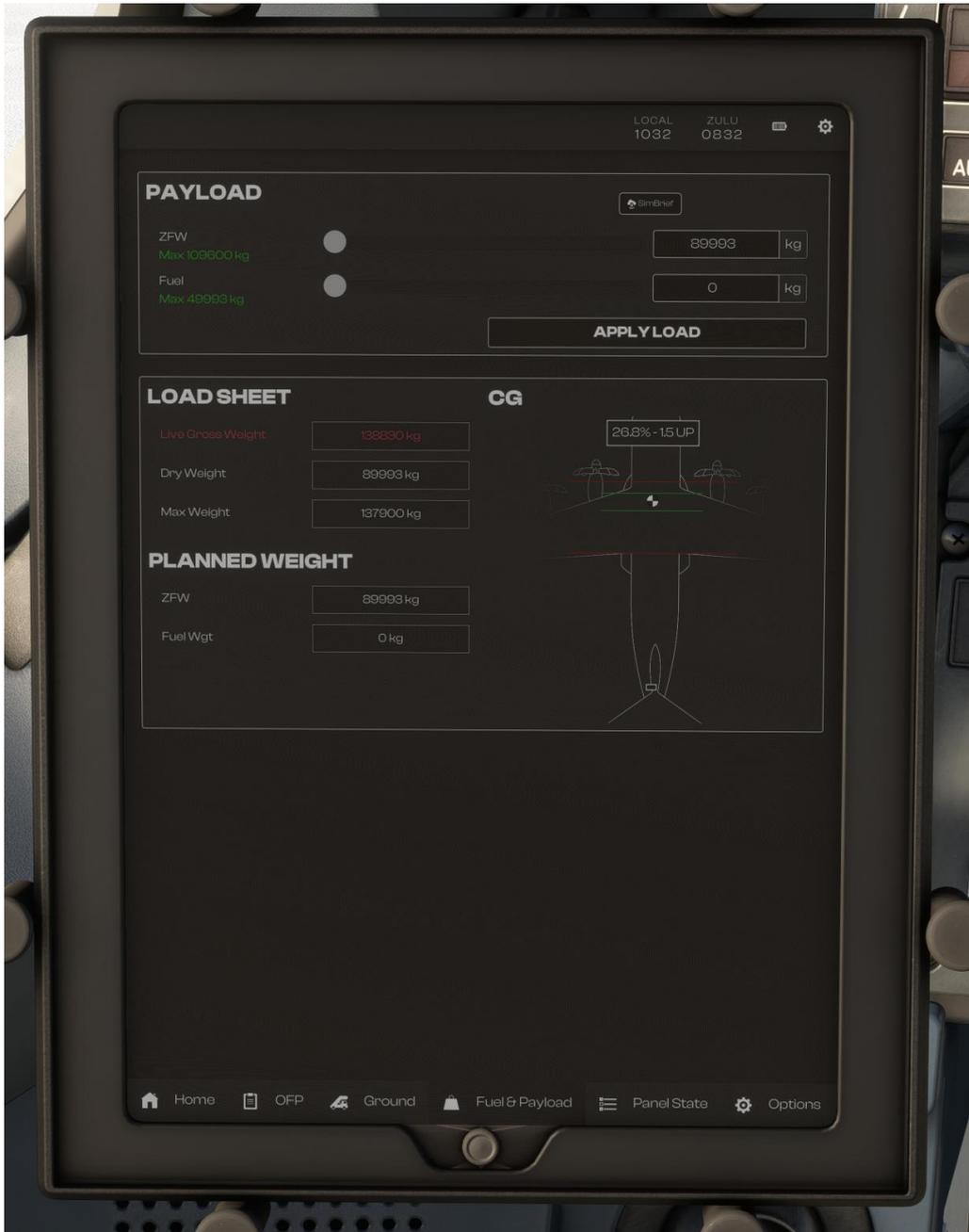
Payload Page – This page allows you to set the fuel and load on the aircraft and apply it to the aircraft.
