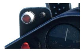
In case of issues with lights, you can use the auditory check button. Once pressed, a continuous sound will be emitted if landing gear is down and locked.
