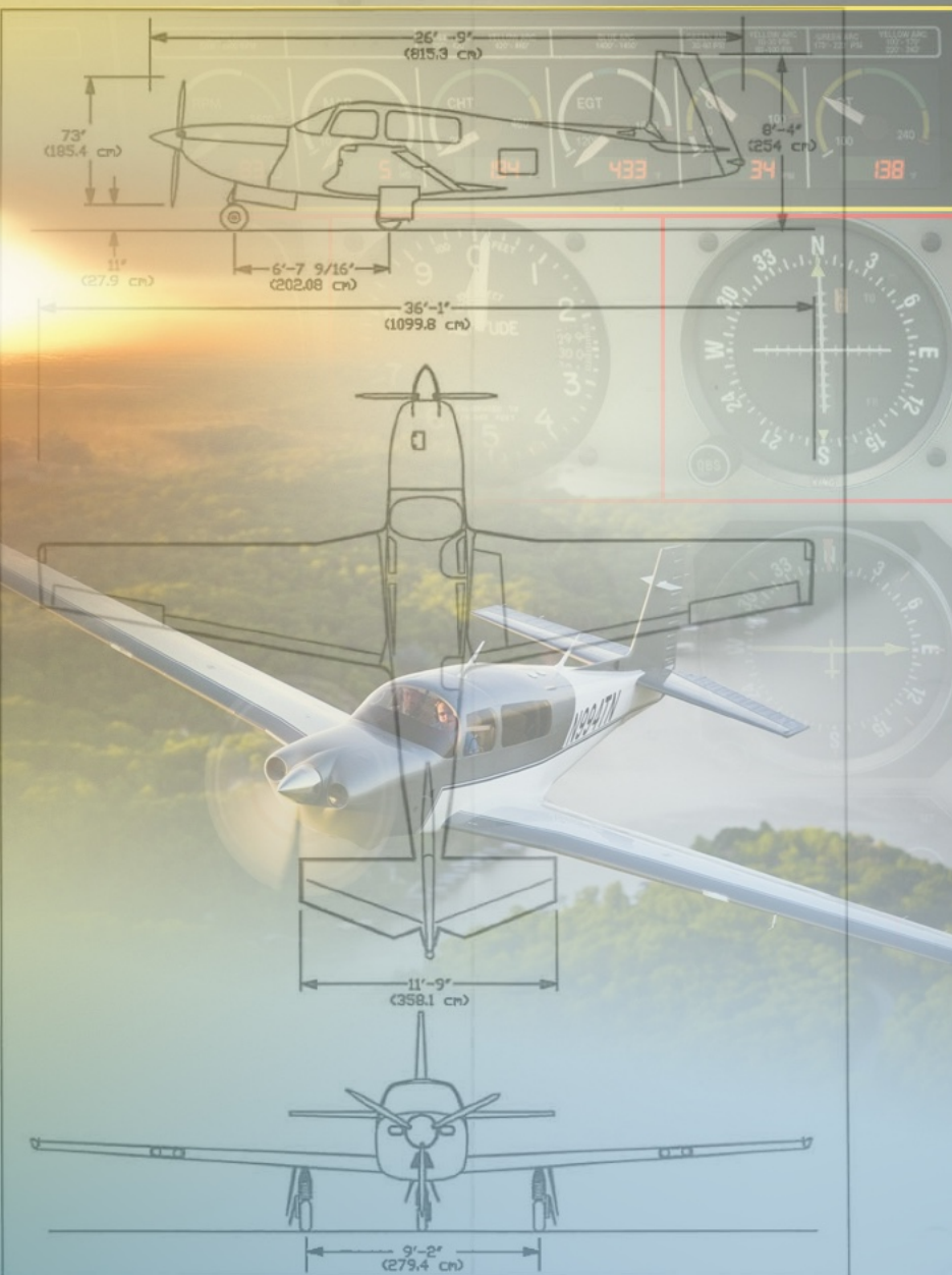
FIGURE 1 - 1 THREE VIEW - M20R
