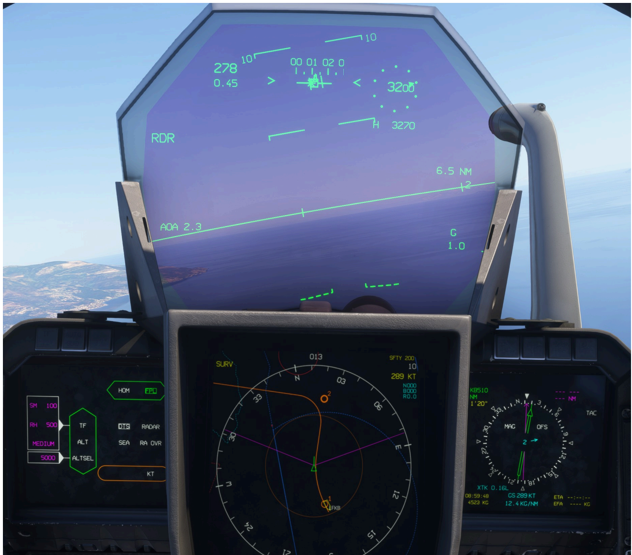
FPL mode active and following the flight plan route
