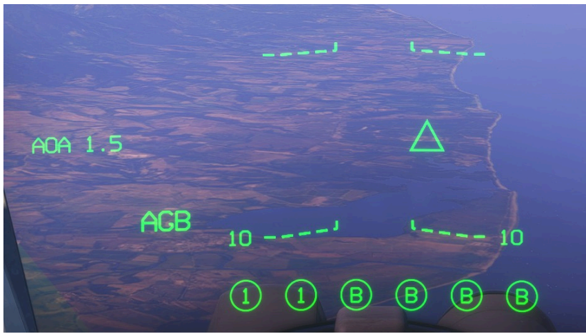
Six bombs carried, with two prepared for release
