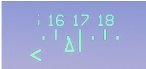
Heading ribbon showing a five-degree deviation
