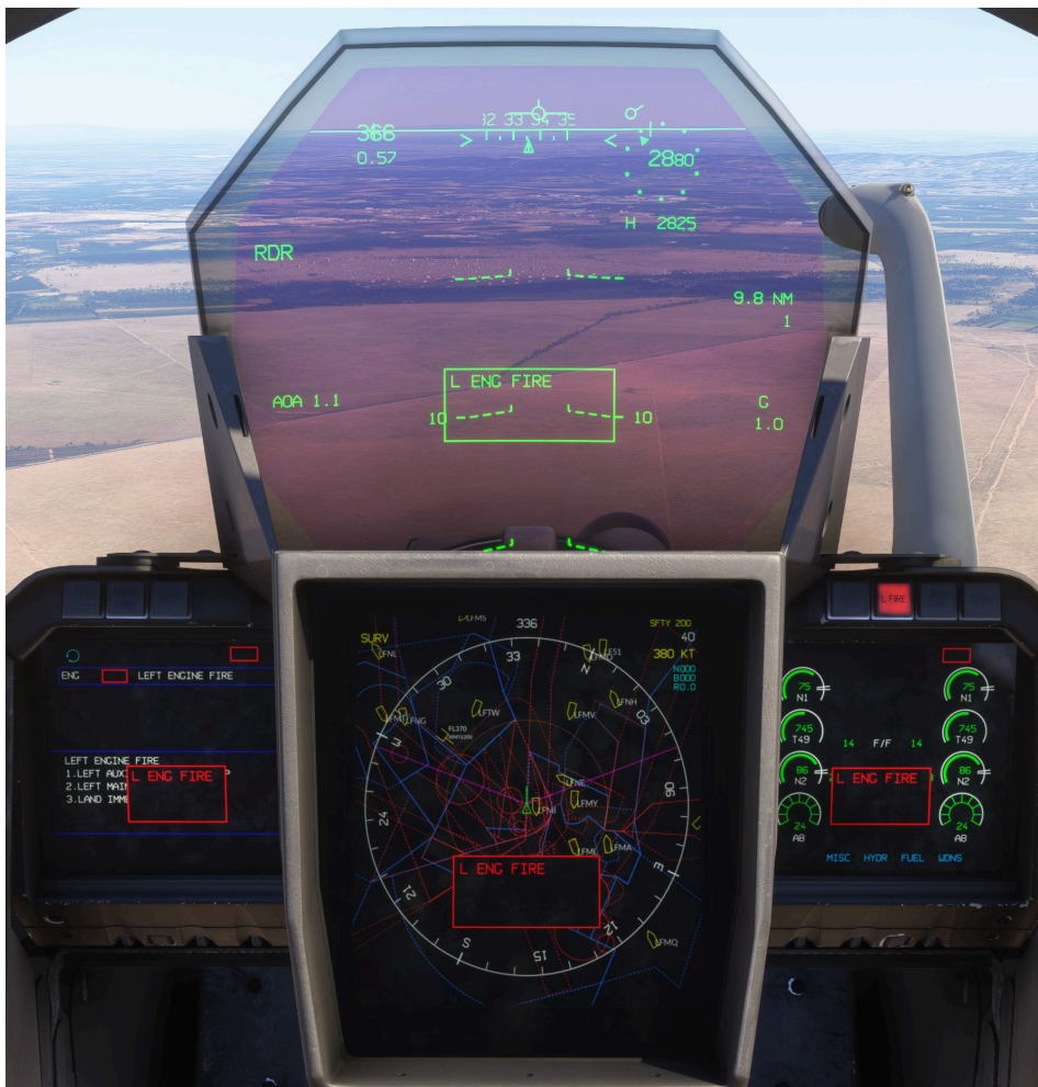
Red alarm displayed on main avionics screens
