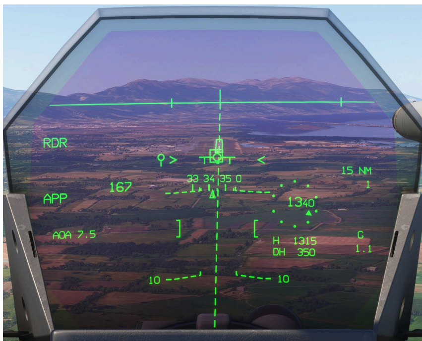
Aircraft established on the correct ILS approach path
