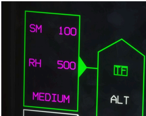
Terrain-following settings on the autopilot page
