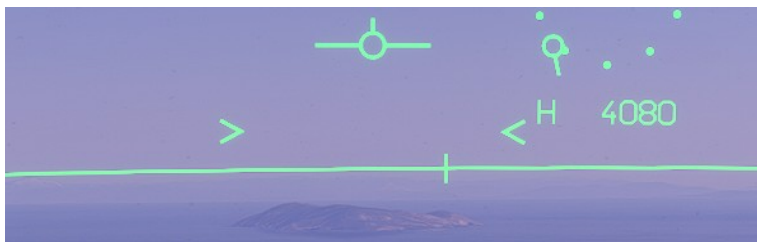
Acceleration brackets indicating a loss of speed
