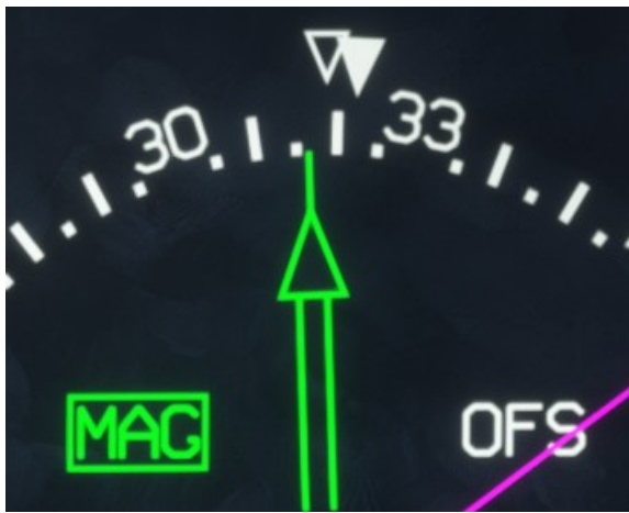
Heading reference set to magnetic
