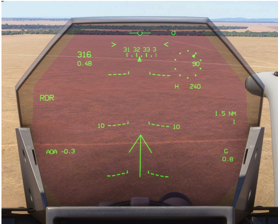
Active safety height alert displayed on HUD
