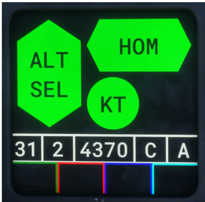
Active ALTSEL mode, HOM and autothrottle in KT mode
