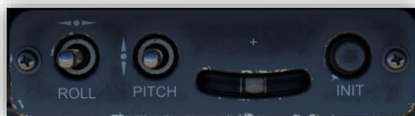
VSD pitch and roll can be offset using momentary switches located below pilot MFD.
