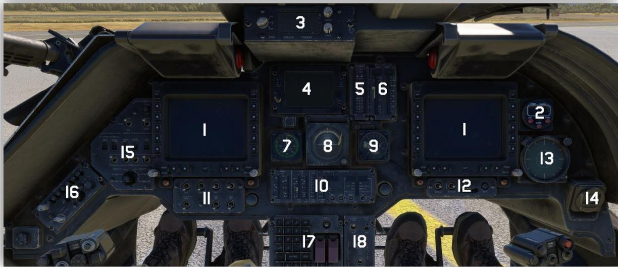
Main instrument panel located in front of pilots consists of multiple instruments, all of which will be usable during each stage of flight. 58D main console integrates both essential standby instruments for basic flight monitoring and advanced Multi-Function Displays (MFDs) for comprehensive navigation and mission planning.
