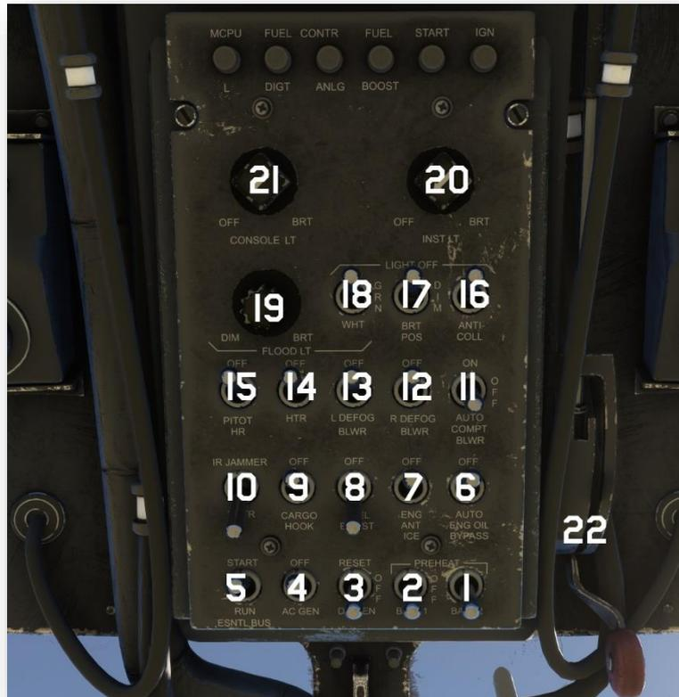
Overhead Panel consists of switches to be used to control base systems of the aircraft like electrical, fuel or lighting.
